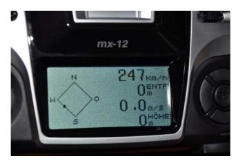
We recommend the handling with the optional Smart-Box. Thereby separate Display-Status indications are possible (see picture). The application of voice output is also extremely reasonably.
